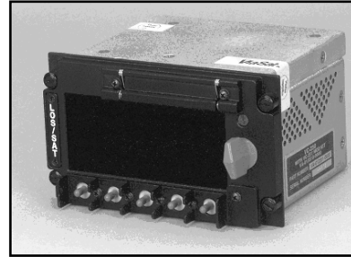
Figure F-1. Control/Fill Panel
